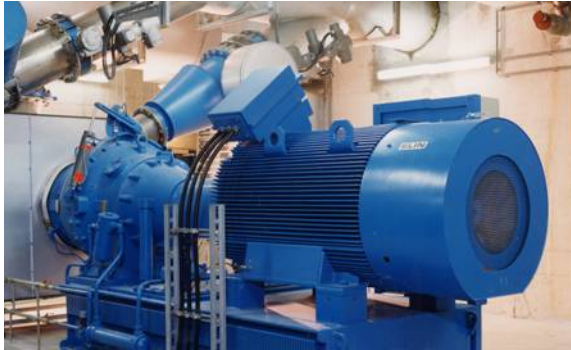
Surface cooled motors 200 kW up to 2,500 kW
